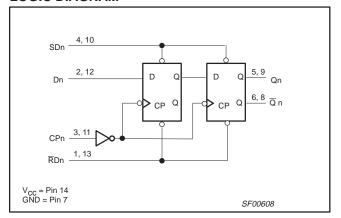
**NOTE:** Data entering the flip–flop requires two clock cycles to arrive at the output.
