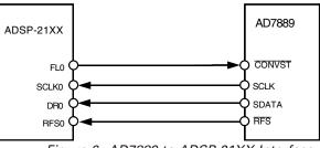
Figure 6. AD7889 to ADSP-21XX Interface
