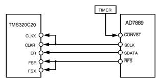
Figure 7. AD7889 to TMS320C20 Interface
