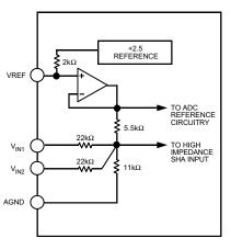
Figure 3. AD7889-1 Analog Input Structure
