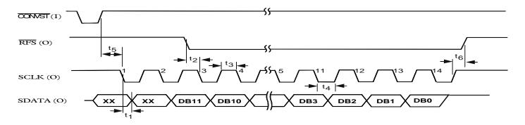
Figure 3a. Mode A Timing Diagram (IDLEHI=1)
