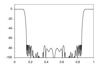
Figure 1b. 4x Interpolating Filter Response
