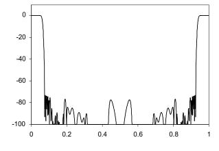
Figure 1c. 8x Interpolating Filter Response
