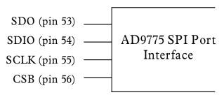
Figure 3. AD9775 SPI Port Interface
