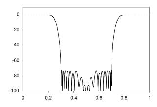
Figure 1a. 2x Interpolating Filter Response
