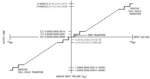
FIGURE 1a. Transfer Characteristic
