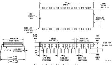
Ceramic Dual-In-Line Package (J) Order Number ADC1242CIJ NS Package Number J28A
