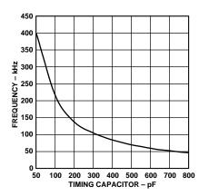
*Figure 5. Frequency vs. Timing Capacitor*
