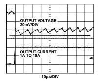
Figure 10. Load Transient Response, 1 A–19 A of Figure 2 Circuit
