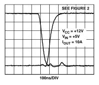
Figure 8. Driver Transition Waveforms
