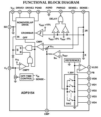
The ADP3154 contains a linear regulator controller that is designed to drive an external N-channel MOSFET. This linear regulator is used to generate the auxiliary voltages (AGP, GTL, etc.) required in most motherboard designs, and has been designed to provide a high bandwidth load-transient response. A pair of external feedback resistors sets the linear regulator output voltage.
