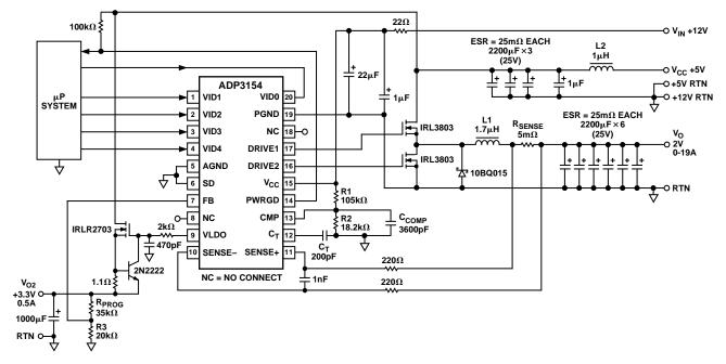
Figure 2. Typical VRM8.2/8.3/8.4 Compliant Core DC/DC Converter Circuit
