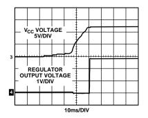
Figure 11. Power-On Start-Up Waveform
