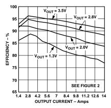
Figure 4. Efficiency vs. Output Current
