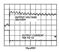
Figure 9. Load Transient Response, 19 A–1 A of Figure 2 Circuit
