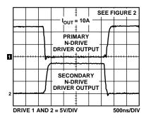
Figure 7. Gate Switching Waveforms
