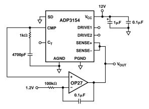
Figure 13. Closed-Loop Test Circuit for Accuracy
