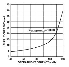
*Figure 6. Supply Current vs. Operating Frequency*
