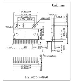
Note) The package of this product will be changed to lead-free type (HZIP025-P-0980B). See the new package dimensions section later of this datasheet.
