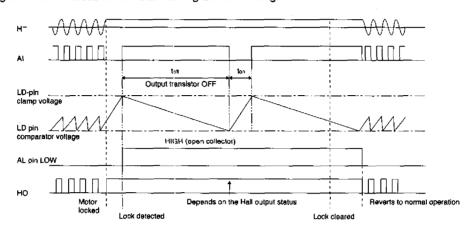
Fig.1 Timing chart for motor locking
