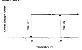
Fig.3 Temperature setting of the thermal shutdown circuit
