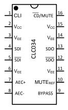
Figure 1. 16-Pin SOIC See Package Number D0016A
