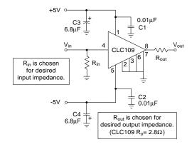
Figure 1: Recommended circuit & evaluation board schematic
