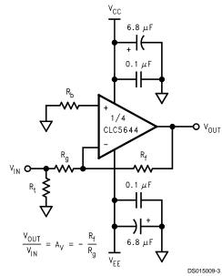
Note:  $R_b$  provides DC bias for the non-inverting input. Select  $R_t$  to yield desired  $R_{in} = R_t || Rg$ .
