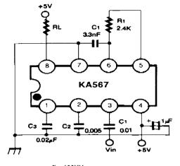
fi = 100KHz Note : Adjust for fo = 100KHz
